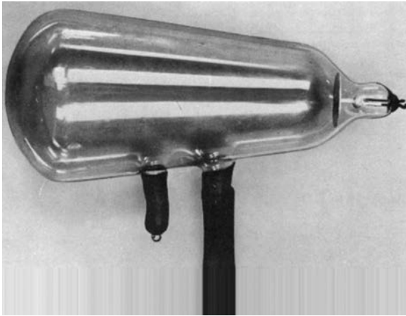
Fig. 1.1 Pear-shaped Hittorf–Crookes tube used in Roentgen’s initial experiments. (Courtesy of Eastman Kodak, Rochester, New York.)
